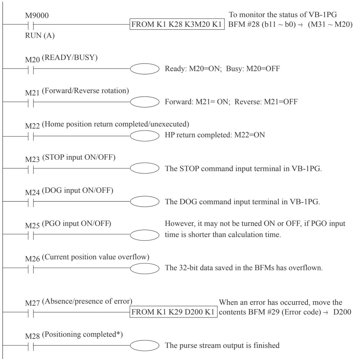
\* When a drive amplifier for a stepper motor without the positioning completed output is used, this signal can be used for recognition of positioning completed and the next operation can be started.
