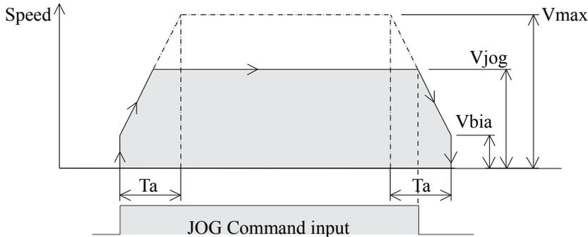
Any value between the bias speed  $V_{bia}$  (BFM #6) and the maximum speed  $V_{max}$  (BFMs #5 and #4) is valid as the command speed  $V_{jog}$  (BFMs #8 and #7). The acceleration / deceleration time  $T_a$  (BFM #15) is the time between  $V_{bia}$  and  $V_{max}$ .
