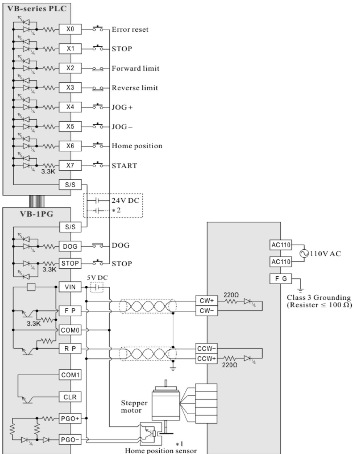
\*1 The number of counts of zero signals is adjusted to 0 (BFM #12, N= 0) when there is no home position sensor.
