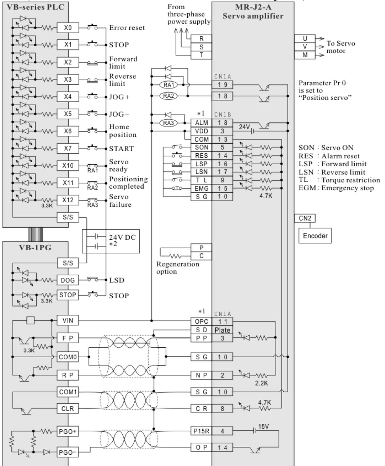
\*1 PIN No. can be modified using the extension parameter. (The example above shows the case where the initial value is set.)
